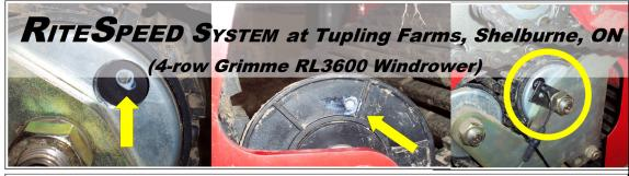
The two pictures on the left show small round magnets embedded in shallow depressions drilled into the flanges of two styles of idler rollers. The third picture shows the sensor on a bracket. It emits a pulse each time the roller makes a revolution and the magnet passes by.
