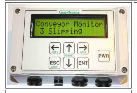
**Controller** with sealed keypad and bright display to navigate the simple menu system for set-up, fine-tuning, and diagnostics. An internal alarm sounds when the pre-set slip percentage is exceeded and the display shows which belt is slipping.
